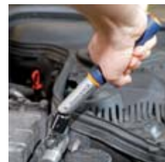
Closure cap and internal locking screw prevent inadvertent change of the setting.
